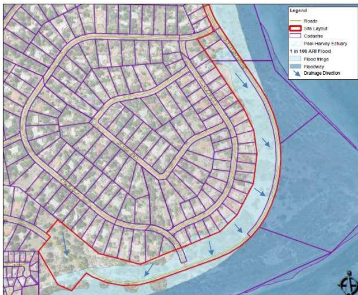
Figure: 100yr ARI flood level
